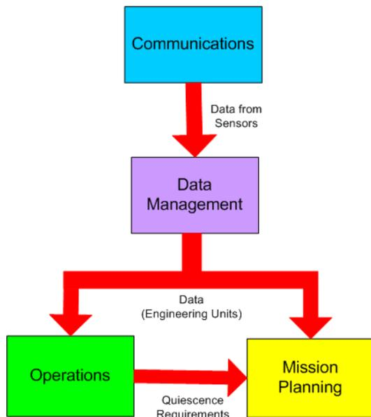
Figure 2: FDMD software modules and information flow.
