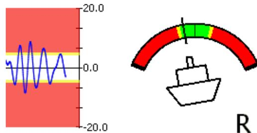
Figure 3: Roll motion history and value indicator in the operations user interface.
