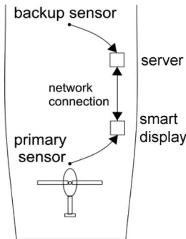
Figure 1: FDMD hardware architecture with backup and error checking functionality.
